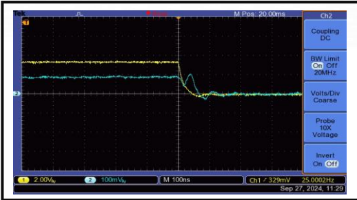
The RF Switch On Time is 100 ns
